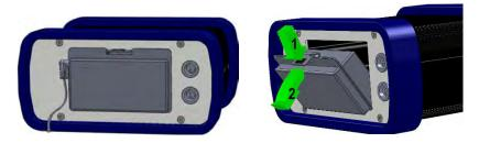
To remove the battery from the device, proceed as follows: 1) Press the burst above to unlock 2) Turn the battery outwards To reinstall the battery, do the same operation in the reversal way.
