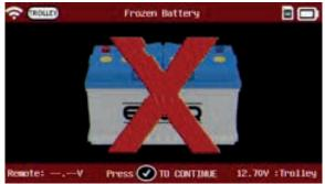
If the battery temperature is too low, (below 32°F / 0°C) the tool will show a battery with an X through it and have an audible chime simultaneously.
