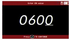
Use the navigating arrows of the keypad to enter the value indicated on the battery (CCA value in this example).
