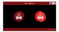
If the battery has been disconnected from the vehicle or is outside of the vehicle, select "Out Vehicle"
