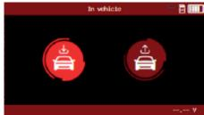
If the battery is still connected in the vehicle select "In Vehicle"
