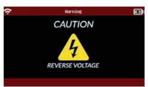
If the battery is connected on the opposite polarity, the screen "Reverse Voltage" will appear.
