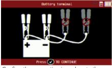
Confirm the connection is as close to the battery terminals as possible
