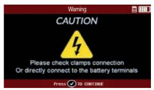
If an issue is found with the connection to the battery, the screen "Please check clamps connection or directly connect to the battery terminals" will appear.
