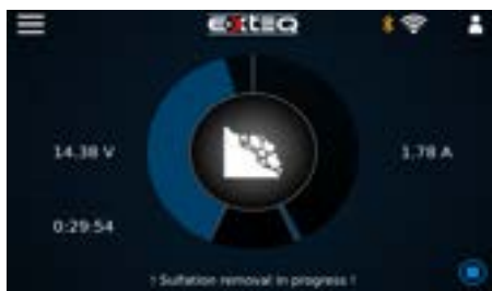
If sulfation is detected the Maximus will try to recover the battery.
