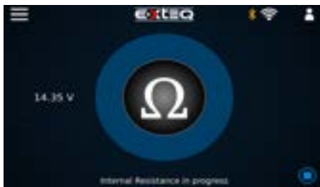
If no pre-charge is needed, the Internal Resistance test will start at this step
