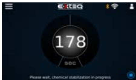
Chemical stabilization after pre-charge finishes.
