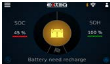
Battery is good but needs recharge
