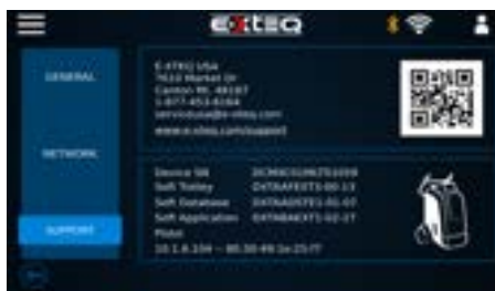
Support icon will display the tool information, and technical support information. The QR code will be available for quick guides.
