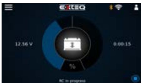
Reserve Capacity test in progress (if needed).
