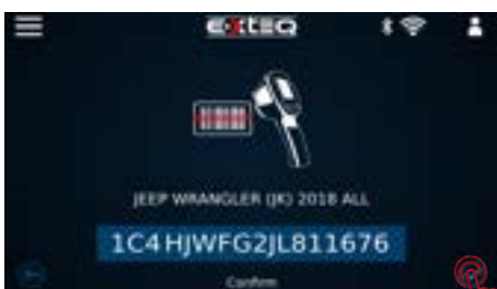
Scan VIN with pistol and VIN will show up on screen of tool
