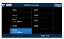
Confirm the Vehicle and Battery information. If battery has been changed, go to the EDIT button and select the correct battery information.
