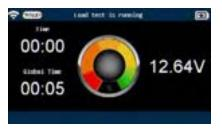
Once the Load Test is done, a graph will display the waveform of the Voltage Drop and Recovery.
