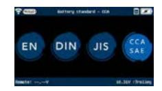
Use the navigation arrows of the keypad to enter the value indicated on the battery (CCA SAE value in this example).
