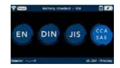
Use the navigation arrows of the keypad to enter the value indicated on the battery (CCĂ SAE value in this example).
