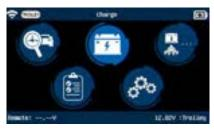
In the "Charge" Icon, the user has the option to select between "Normal Charge mode" (40A) and "Fast Charge Mode" (80A/100A).
