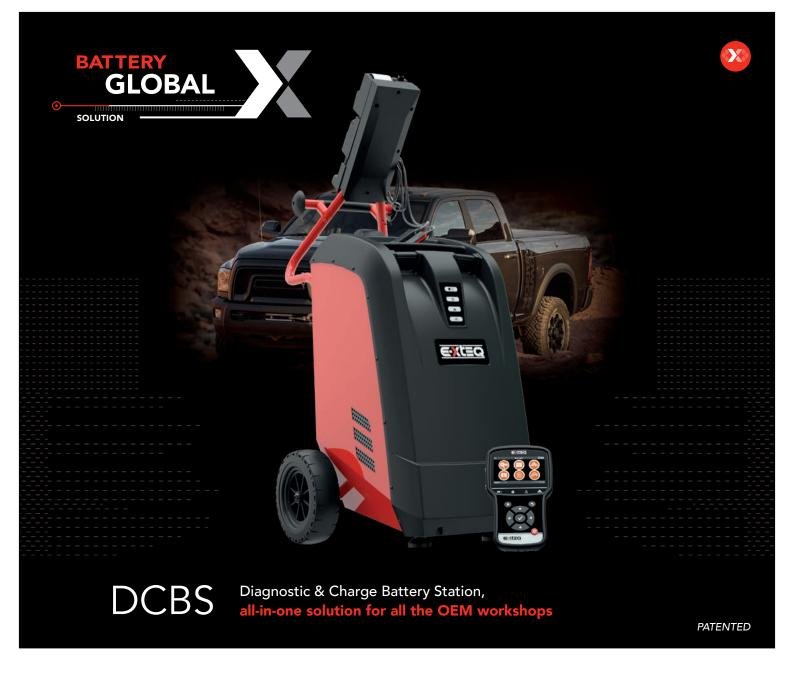
All-in-one solution with a built-in 12V/100 Amp battery charger/maintainer that provides in-depth features and functions to stabilize battery voltage during ECU reflashing and is capable of charging batteries regardless of chemistry. Remote and its handheld diagnostic tester that can be used simultaneously are both equipped with their own temperature sensors battery cables.
