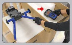
Connect the cables between docking station and trolley.
