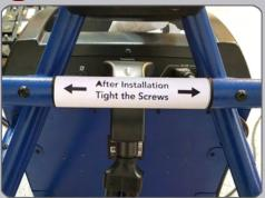
Mount the trolley and remote cable hooks with the 5M - 10mm screws.
