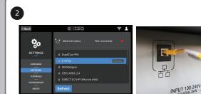
The first time the MB1550 is ON, an internet connection will be prompted. LAN or Wi-Fi connection will be the options. RJ45 port can be found on the rear panel. NOTE: LAN connection is recommended for automatic update.
