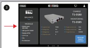
Based on the monitoring cable connected, the MB1550 will automatically select the correct module. Verify by part number that the correct module was selected.
