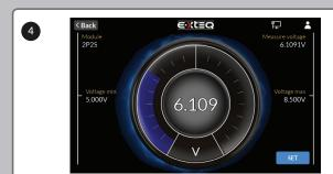
Once the module is selected the screen will display the current voltage of the module.
