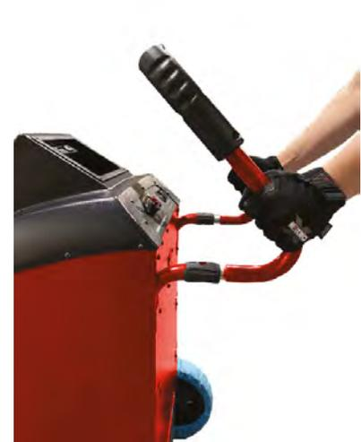
3. Attach the handle to the trolley using the included 6M-35mm screws and nuts.
