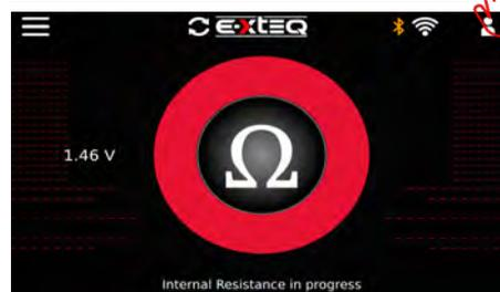
Internal Resistance test in progress
