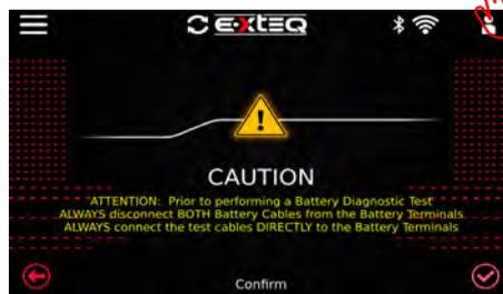
Warning screen to test battery on bare terminals
