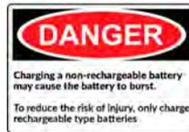
The battery contains chemicals that may generate explosive gases. Before handling the battery, remove all metal accessories such as rings, bracelets and necklaces. Short circuit at battery terminals may cause burns. Do not place batteries near flames or other heat sources
