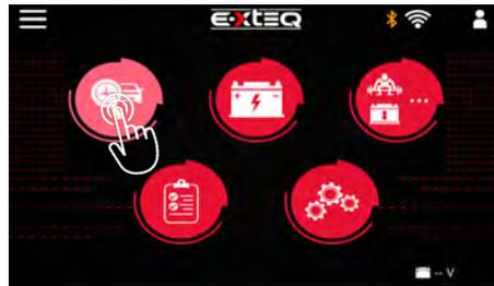
To run a diagnostic, select the first icon labeled "DIAGNOSTIC", then follow vehicle or manual battery selection (listed above)
