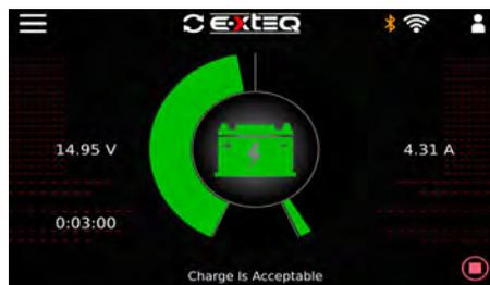
Top off charge is acceptable Test can be stopped manually
