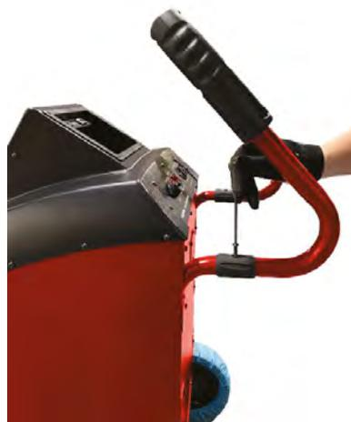
4. Mount the trolley cable hooks with the included 5M-10mm screws.
