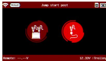
If the terminals are not accessible, select Jump Start Post (limits the current injected into the chassis to 40A).
