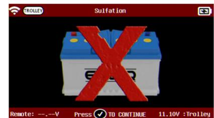
If an issue is found with the battery, the tool will show a battery with an X through it.
