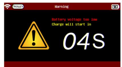
If the battery voltage is too low, the tool will perform a pre-charge on the battery, and then continue with the diagnostic test.
