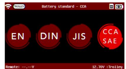
Use the navigation arrows of the keypad to enter the value indicated on the battery (CCA SAE value in this example).
