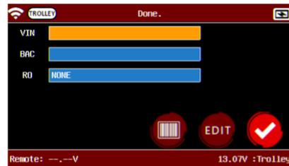
BAC should be pre-filled. VIN will also be pre-filled (requirement to start test).
