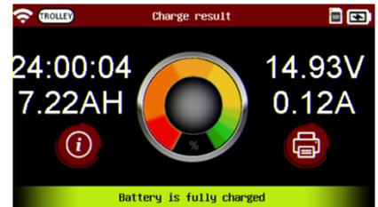
After 24 hours of charge (or<0.2A) with no issues, the Charge result will come back as "Battery is fully Charged".
