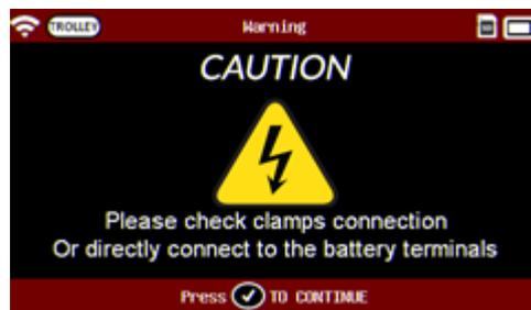
If an issue is found with the connection of the battery, the screen "Please check clamps connection or directly connect to the battery terminals" will appear.
