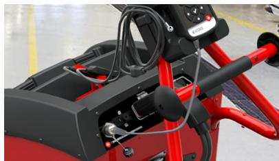
5. Ensure the Ethernet Cable is connected to the trolley and remote as shown
