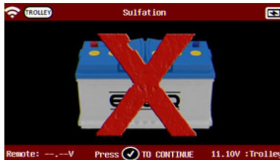
If sulfation is found on the battery, the tool will show a battery with an X through it and audible chime simultaneously.
