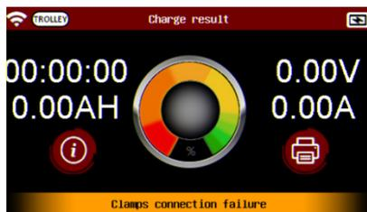
If the clamps are not detecting the battery correctly, the result will come back as "Clamp Connection Failure" and the test must be performed again.
