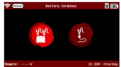
Select battery terminal if they are accessible. (For Diagnostic, it is always recommended to test at bare battery terminals for most accurate results).
