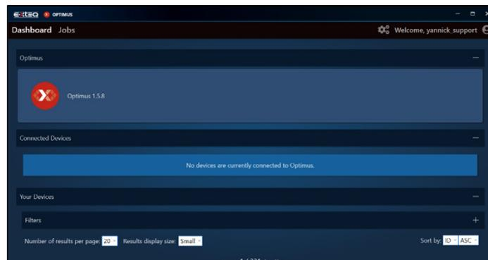
When connecting your tool, it will appear in "Connected Devices". All the recorded job files will be transferred automatically.
