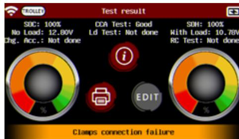
If the test is interrupted, or the clamps are not detecting the battery correctly, the result will come back as "Clamps connection failure" and the test must be performed again.
