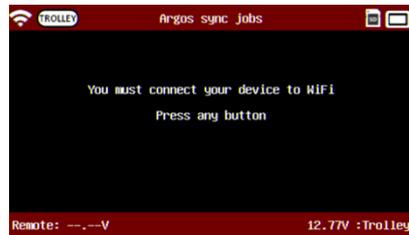
If you are not connected to Wi-Fi (Remote to Network), there will be a message displayed. Please follow the steps indicated in the section "Wi-Fi Connection (Remote to Network)" in this manual.
