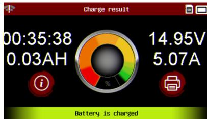
If the charge finishes with no issues, the tool will show "Battery is Charged".
