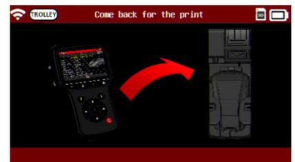
After Complete Diagnostic has been performed, go to the print icon to print the receipt of the result. Remote has to be replaced in the Docking Station to print.
