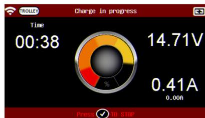
The tool will automatically perform a charge on the selected battery and the Remote will display the charging information.
