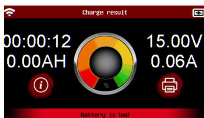
After pressing the ✓ Button, the results will display showing the charge result as "Battery is Bad"
