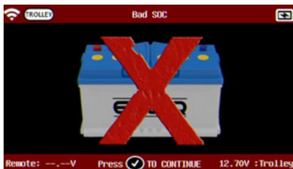
If a wrong value on the battery type is detected, the tool will show a battery with an X through it and have an audible chime simultaneously.
