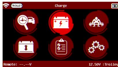
In the “Charge” Icon, the user has the option to select between “Normal Charge mode” (40A) and “Fast Charge Mode” (80A/100A).
