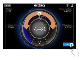
Click the center of the gauge where the value is displayed, a keypad will display to input the exact value. Confirm the value by taping "Ok".
