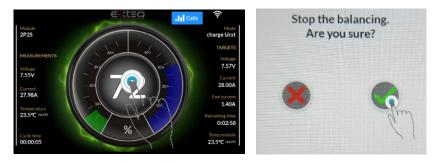
Tap on  $\checkmark$  button, to confirm the termination of the process. Balancing will stop and the lid will open after operator confirms.
