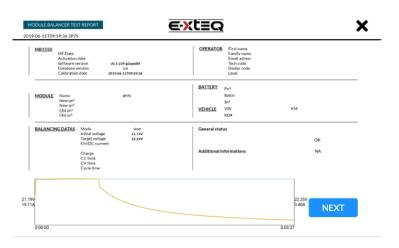
The module balancer stores the balancing reports in the internal memory. They are downloadable through USB port.
