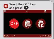
NOTE: The Trolley and Remote will now communicate only through the physical connection between them. To check if the connection is working, connect to a battery and see bottom of remote to see if the trolley is reading voltage.
